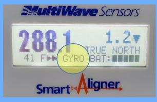
1. If GYRO appears on the Tool's measurement screen, it has lost the GPS compass solution. While the internal Gyro helps maintain a solution in this event, the azimuth measurement will not be accurate.
