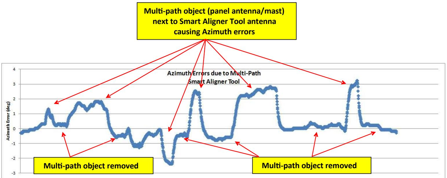
As can be seen from the graph above multi-path can cause a positive or negative error to the azimuth depending on where the multi-path object is placed. Therefore it is very important to have the Tool GPS receiving antennas extended away from the antenna to be aligned. The Smart Aligner Tool extends the GPS receiving antennas away from the antenna to be aligned in order to eliminate the errors as seen in the graph above. See image below.
