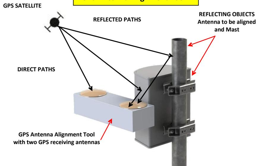
The error caused by multi-path is dependent on the GPS satellite geometry, so that in some cases, the error may be negligible, but in other cases, it can be up to 3° or more. As can be seen from the images above, one of the GPS receiving antennas is receiving a signal from the GPS Satellite that is reflected off the mast and antenna to be aligned. The path of the reflected signal is longer than the direct path, resulting in an azimuth error.
