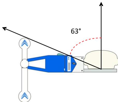
**Smart Aligner mounted to back of antenna with the GPS receiving antennas extended to mitigate RF and multi-path**
